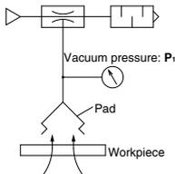
**Exercise:** Using a supply pressure of 0.45 MPa, when the ejector (ZH07□S) picks up a workpiece that leaks air, the vacuum gauge indicated a pressure of -53 kPa. Calculate the leakage volume from the workpiece.
