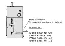
Option symbol With a timer controlled solenoid valve type auto drain (applicable to moderate pressure)
